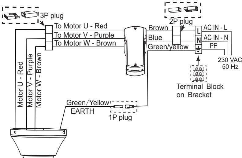
Connect the plugs as shown in the picture and connect the mains voltage at the terminal block.
